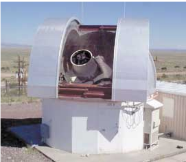
1 METRE TELESCOPE OF LINEAR, New Mexico. The telescope, one of two on the site, is equipped with advanced CCD detectors and high speed computers. It operates automatically and sends data to the Lincoln Laboratory at MIT for checking and transmission to the Minor Planet Center. LINEAR has discovered more Near Earth Objects of diameter greater than 1 kilometre than any other system so far.
