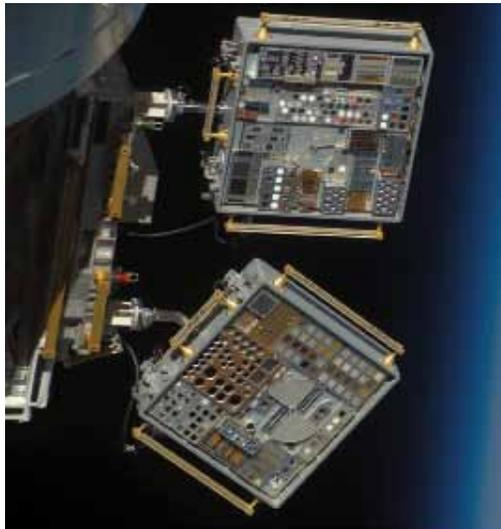
**It's been eight years since the first Materials International Space Station Experiment, or MISSE, arrived at the orbiting laboratory. During that time, more than 4,000 materials samples have been placed outside the space station to test how they react to the harsh environment of space.**
