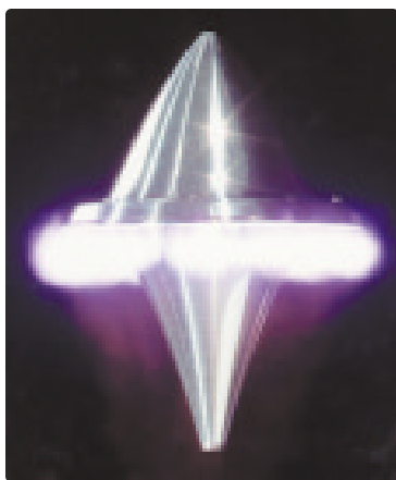
A model of a lightcraft, illuminated from below by a laser beam.
