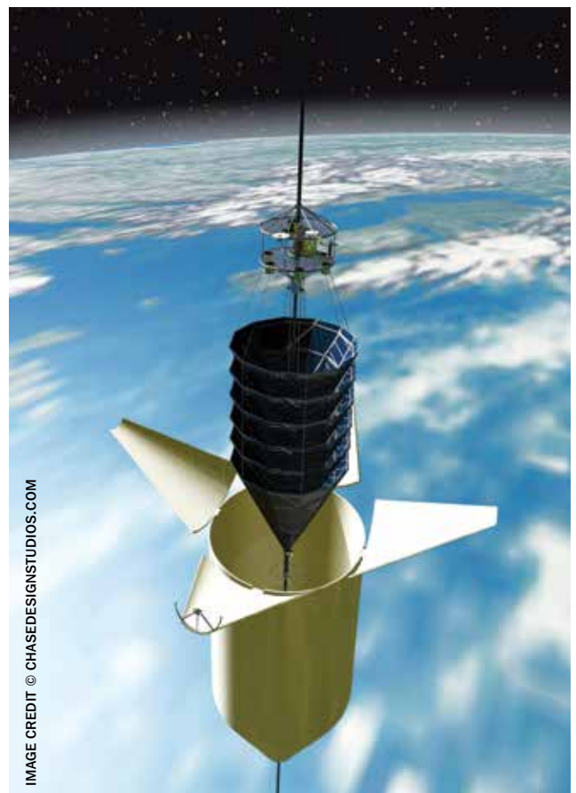
The tether climber is exiting its protective box above the atmosphere and is preparing to deploy its solar cells to initiate power for the climb to GEO and beyond.
