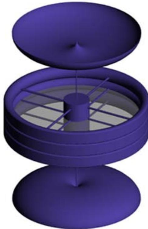
**Figure 10 - Expanded Vademecum with micro-gravity center, twin mirrors and solar panels**
