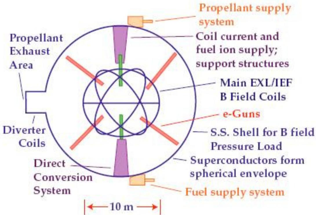
**Figure 6 – Schematic outline of DFP engine system**
