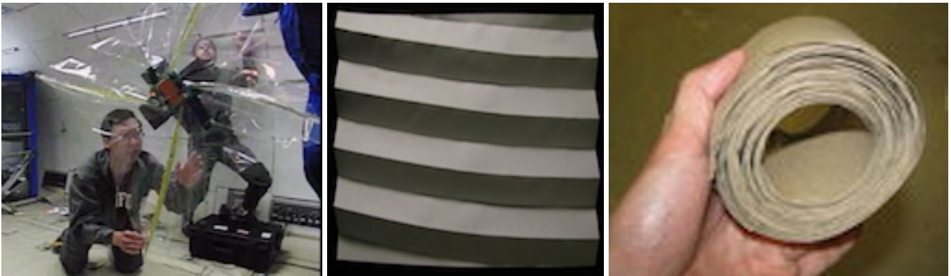
Left: deployment on Zero-G Flight Right: special way solar sail is folded to fit inside 10x10x cm cube sat
