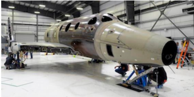
Virgin Galactic's 2nd SpaceShipTwo under construction in Mojave, California
