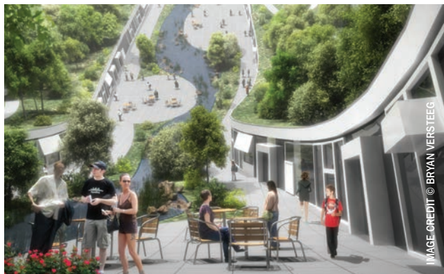
Artist concept of a small early space settlement. Note the curvature necessary to generate pseudogravity by rotation.
