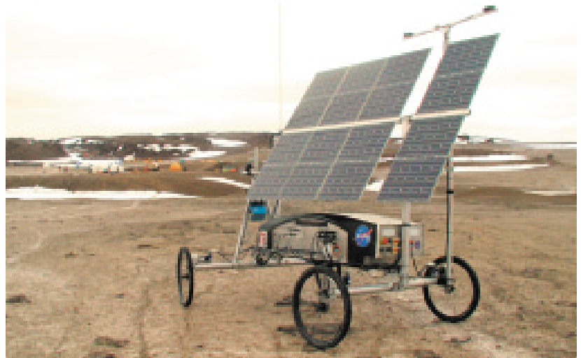
Carnegie Mellon University's autonomous sun-following Hyperion rover during field testing on Devon Island in Summer 2001.
