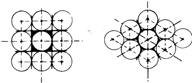
Fig. 2. Two close-packing options for circular modules.
