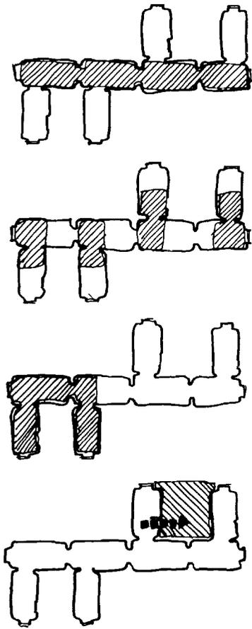
Fig. 12. Schematic plan of functional options for branching.
