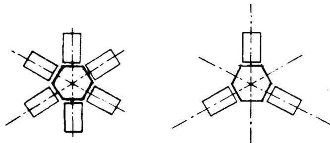
Fig. 3. Plan view of multiple coupling techniques.
