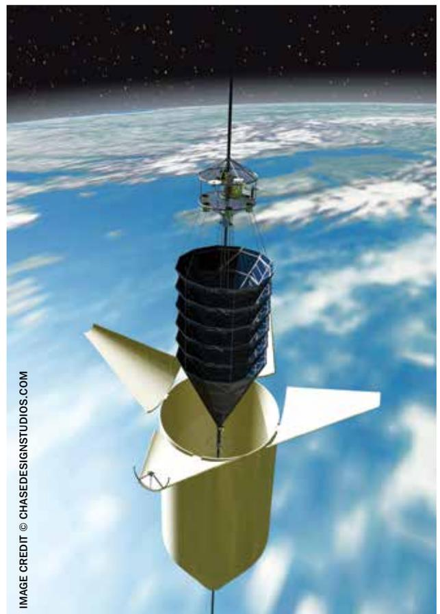
The tether climber is exiting its protective box above the atmosphere and is preparing to deploy its solar cells to initiate power for the climb to GEO and beyond.
