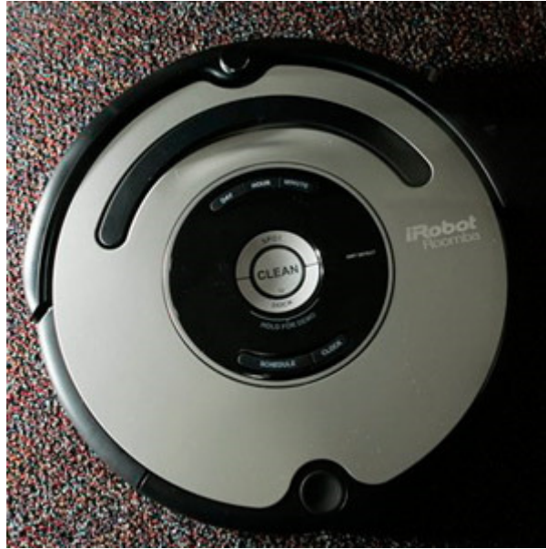
Fig. 87. The Roomba is a robot that can vacuum the house
