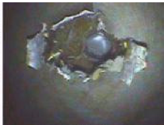
Fig. 11. STS-118 radiator impact damage. The ingress hole is 10mm in diameter, but the exit hole is much larger and very irregular. This is typical of all penetrating impacts.
