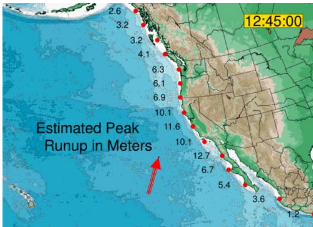
Figure 7. Peak run-up wave heights on the North American Pacific coastline based on a simulated ocean impact of asteroid 2004MN4. Simulation results courtesy of Dr. Steven Ward, Institute of Geophysics and Planetary Physics, University of California, Santa Cruz, CA.
