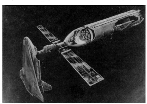
SPACE PLATFORM -- An artist's drawing shows the Space Shuttle's external tank in Earth orbit as the first step of a space platform. A crew of three would inhabit the forward area and construct additional living and working space in the remaining volume (17,500 cubic feet) of the liquid oxygen propellant tank.
