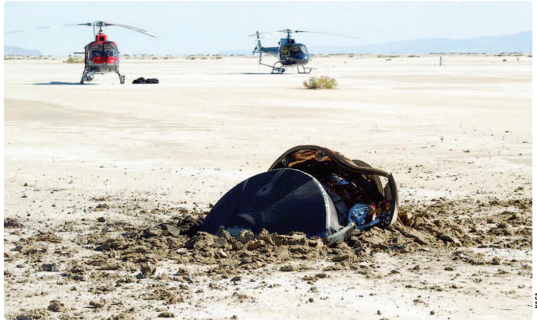
The Genesis spacecraft slammed into the desert floor after a failed parachute return to Earth.
