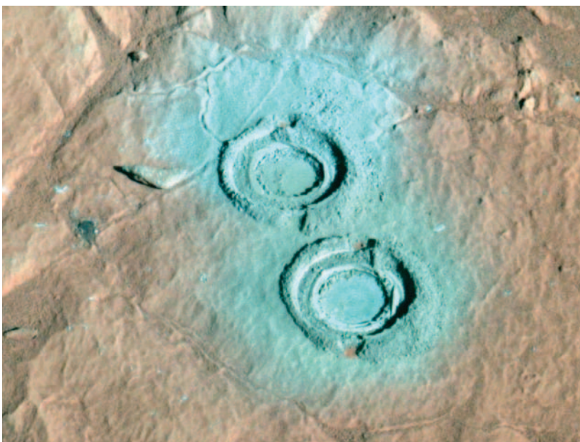
Spirit looks at two holes it carved into the rock "Clovis," located on the west spur of the Columbia Hills. The rock exposed in the Columbia Hills is lighter in tone and is softer than that which was examined out on the plains of Gusev Crater.
