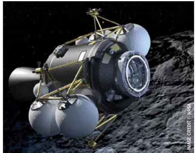
This image shows a single-stage, dual thrust-axis lunar lander with "ut-rigger" hypergolic propellant tanks.
