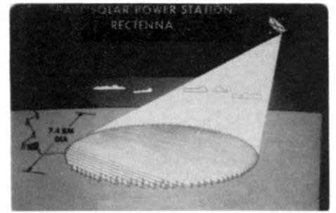
309 Rectenna configuration for receiving microwave transmission from SPS.
