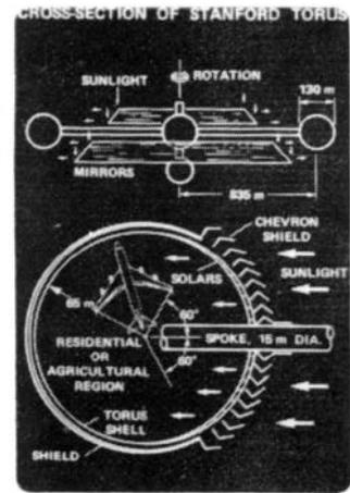
226 Details of the Stanford Torus design -- cross-section.
