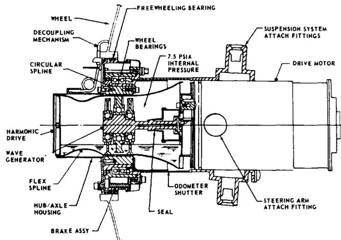
Fig. 8. Traction drive assembly.
