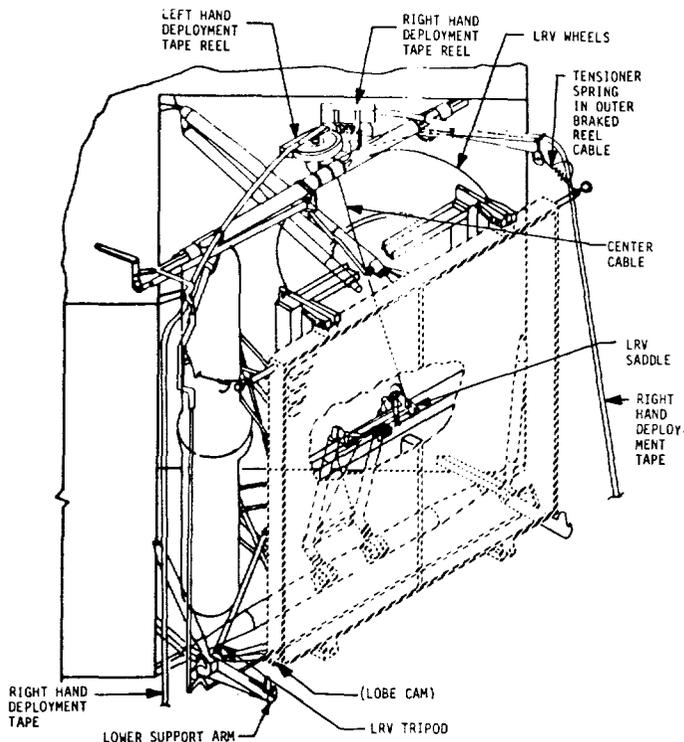
Fig. 21. Lunar module/space-support equipment with LRV installed.
