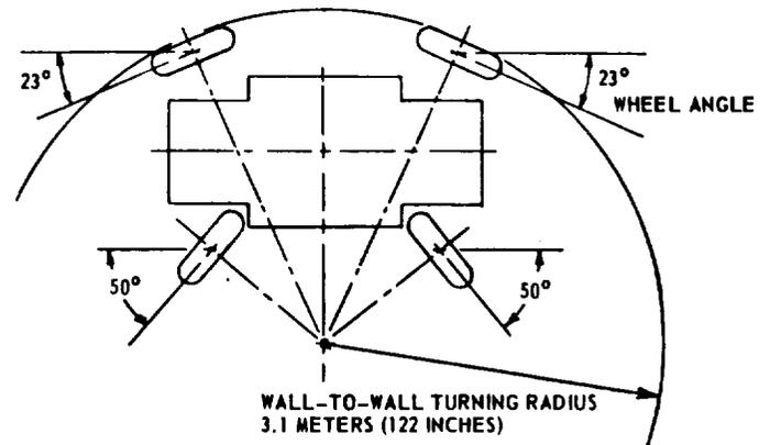
CAPABILITY VERIFIED BY ACTUAL MEASUREMENT ON QUAL AND FLIGHT #1 VEHICLES
