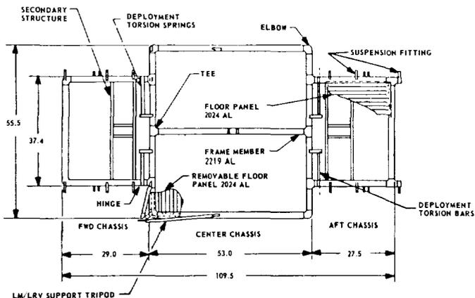
Fig. 5. Lunar Roving Vehicle chassis.
