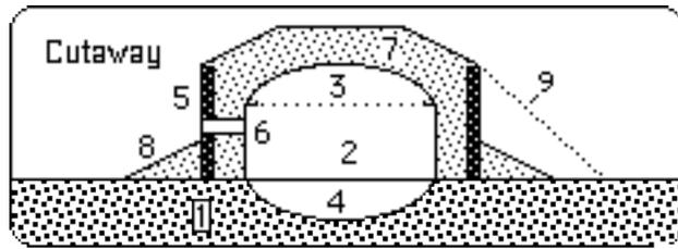
In the illustration above, (9) represents the slope of the moon dust shielding mound if a retaining wall were not used. Now in  $1/6^{\text{th}}$  gravity, the weight of the retained moon dust might not exert enough pressure to topple a well-built brick wall. Experience will tell, however.
