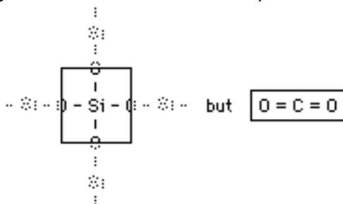
Actually, the hydrides of Silicon behave more like those of boron (with a +3 valence) than those of carbon. The two (Si, B) are similarly very reactive to oxygen, water, and the halogens (chlorine, fluorine, etc.) Even in compounds where they each (Si, C) form only single bonds there is this significant differences. Silicon bonds poorly to itself as a basis for polymer building.
