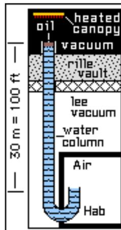
The weight of column of water 30 meters or 100 feet high exerts enough counter-pressure to keep habitat atmosphere at 0.5 Earth normal (42% O<sub>2</sub>, 58% N<sub>2</sub>) pressure from flowing out the open ended J-shaped tube.
