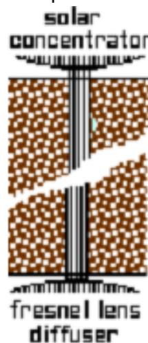
The five 60 mm (2 3/8") bore holes through the tube roof-ceiling could be used to drop in miniaturized survey equipment designed to demonstrate how we can robotically map the interior of lunar lava tubes, profiling their complex shapes and cross-sections. These tests finished, the bore holes could be filled with fiber optic bundles to let in sunlight concentrated up to thirty times. One bore hole could be used for communications access
