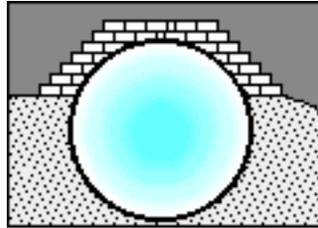
However, this form of shielding can only be constructed after the habitat module is in place.
