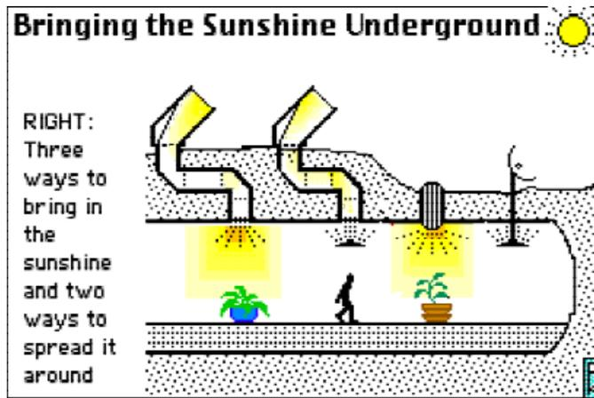
Now the sunlight tubes in the Terra Lux home, were straight shafts. We would need to design them in zigzag pattern for use on the Moon, so as to avoid a pathway for cosmic radiation into the living space. A straight path option that would work would be a solid optic fiber bundle.
