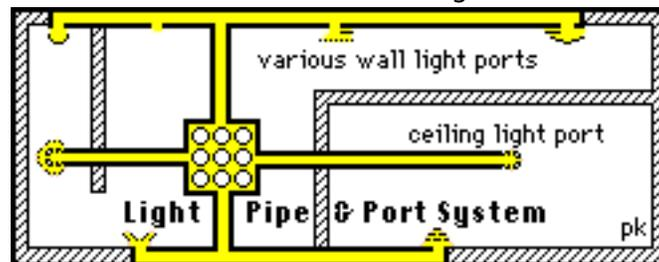
The recent development of Light Pipe technology suggests an altogether different approach to indoor lighting on the Moon. Instead of a multiplicity of individual lamps and light fixtures, a network of Light Pipes whose rib-faceted inner surfaces channel light without appreciable loss to locations remote to the light source could be built into each building, ending in appropriately spaced and located Light Ports.
