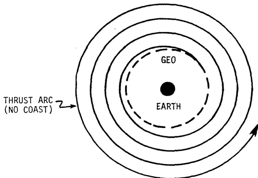
(a) CONTINUOUS THRUST SPIRAL TRAJECTORY MODE
