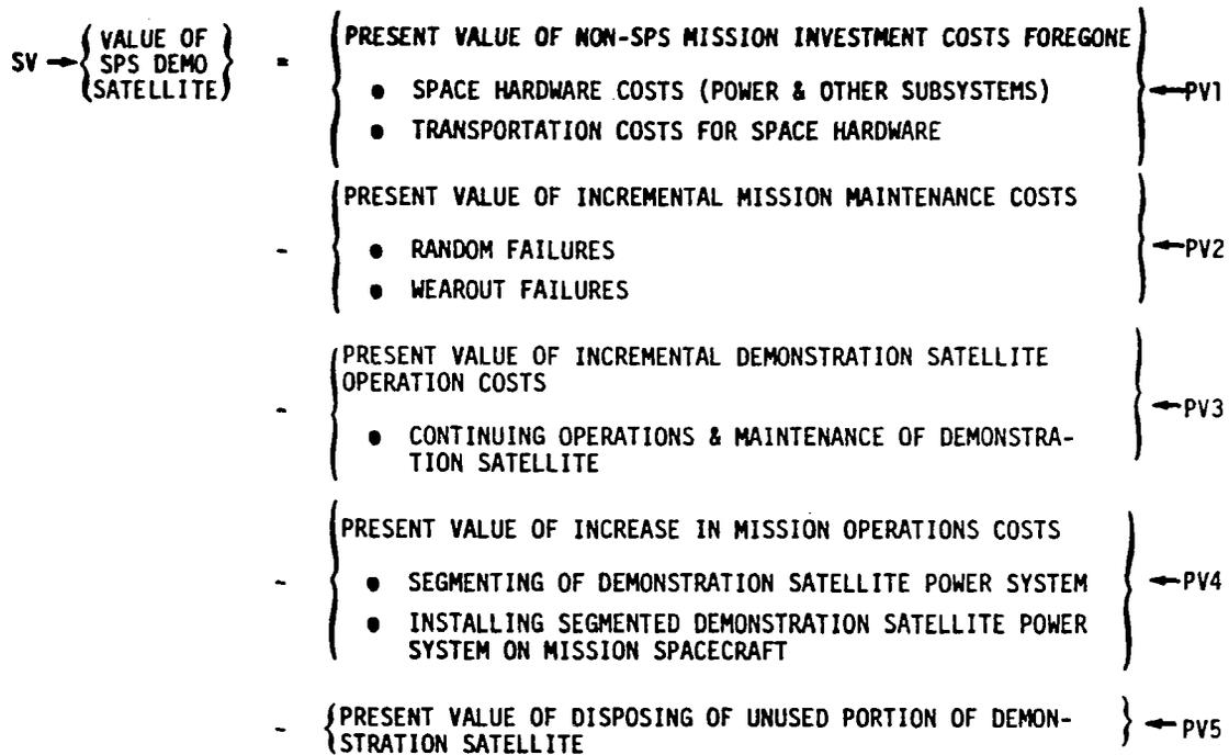
FIGURE 3.6 SALVAGE VALUE--SPS DEMONSTRATION SATELLITE USED AS A SOURCE OF POWER AND OTHER SUBSYSTEMS FOR OTHER ACTIVITIES
