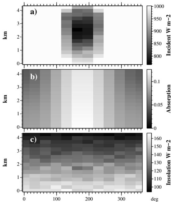
Figure 6: Incident photon power density above the blinders (a), effective absorptivity of the blinder-equipped settlement surface (b), insolation below the blinders. All are as function of the cylindrical coordinates  $\varphi$  and  $z$ . In (a), values over 1 kW are shown are white.
