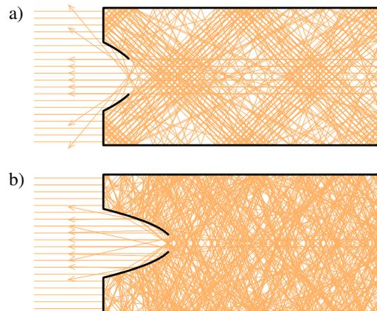
Figure 1: When sunlight is concentrated into a light channel by a parabolic concentrator, photons can only escape through the same slit where they entered. Light intensity inside the box in case (b) is higher than in case (a) because the concentration ratio is higher.
