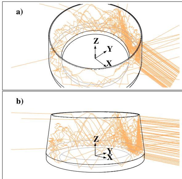
Figure 7: Photon paths inside the light channel from two viewing angles. A vertical sheet of input photons enters from the right hand side and propagates along  $-\hat{x}$  at  $y = R/2$ , while  $z$  is a random number in interval  $[0, Lz/2)$ .
