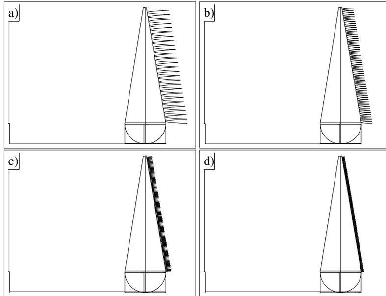
Figure 5: 2-D cuts showing the parabolic concentrators for different slit half-width parameters  $p$  of 4 m (a), 2 m (b), 1 m (c), 0.5 m (d). The value  $p = 1$  m (panel c) is used in the calculations. In the limit of small  $p$  (small and numerous concentrators), the parabolic concentrator zone looks dark and featureless to an external viewer, as was depicted in Fig. 3.
