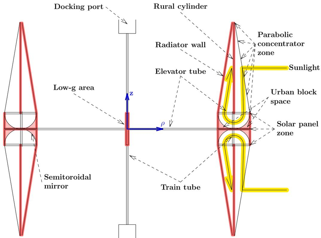
Figure 4: 2-D cut view of the cylindrical space settlement. Thick radiation shielding parts of the walls are shown in red.
