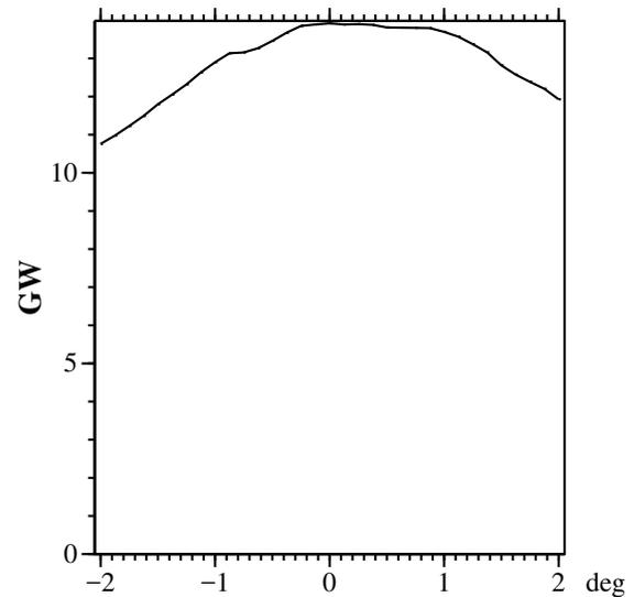
Figure 8: Power absorbed by the living cylinder as function of sun angle.
