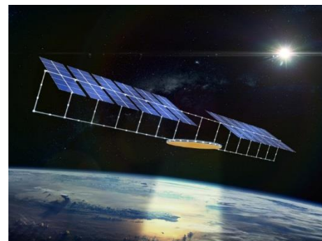
Figure D-20 — Multi-Rotary Joints SSP
