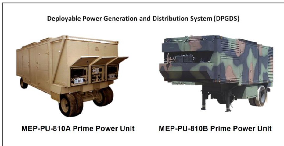
Figure 6-1 – The MEP-PU-810 generator, rated for 840 kW output, consumes 60 gallons (180 kg) of JP-8 per hour [75]
