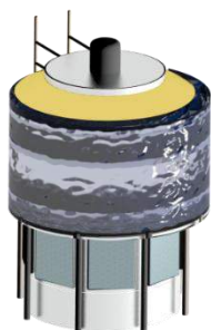
Figure 3.3.5: Water Storage Tank
